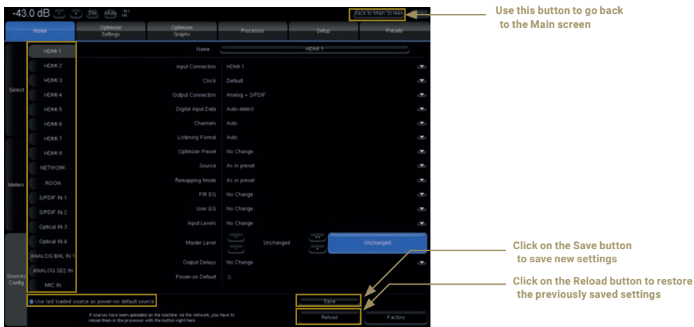
Figure 33: Source Configurations panel
